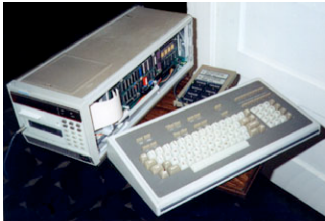
Tek 4041 BASIC Language 68000-based Computer Disguised as Electronics Instrument
